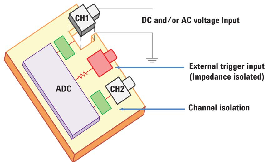
Figure 2. Isolated channel scope block diagram.
